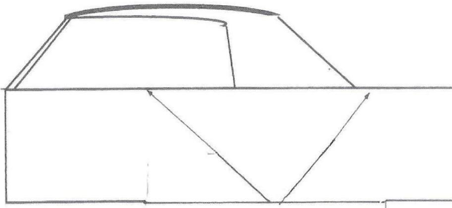
Interior slope allows 4 inches front to rear. Interior will be flat across. If front half of interior has no slope this allows only 2 inches of slope for the rear half. If the front 3/4 of the interior is flat then that leaves one inch for the remaining 1/4 of the interior.
